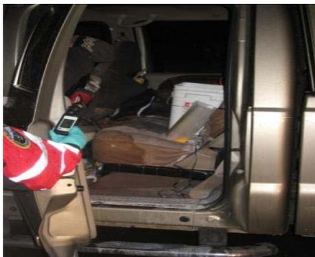
HM7 monitors detected dangerous readings at the gaps of the truck doors, even when closed. Levels inside the vehicle triggered high alerts on the 4 gas monitor. *Note that H<sub>2</sub>S will deaden your sense of smell at about 150 ppm, masking estimates of the on scene danger.*
