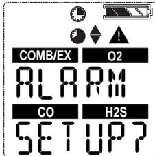
Figure 3-4 Alarm Setup
