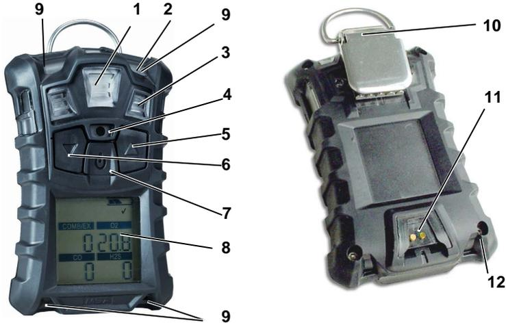
**Figure 2-1 Instrument view**
