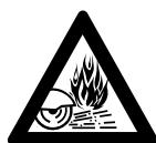
Sparks from cutting metal can burn or cause clothing to catch fire. Always direct sparks away from the operator or any flammable surroundings. Never cut metal while standing on a flammable surface, such as wood or tar paper. Where there is a risk of fire, have appropriate fire extinguishing equipment readily available.
