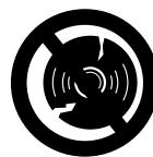
Inspect the abrasive wheel frequently and replace immediately if the abrasive wheel is cracked or warped. Cracked or warped wheels may shatter or break and cause serious or fatal personal injury. Out-of-round or unbalanced abrasive wheels increase vibration and reduce the service life of the cut-off machine.
