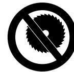
Never use circular saw blades, carbide tipped blades, rescue blades, wood-cutting blades or toothed blades of any nature. They can cause severe personal injury from blade contact, thrown objects and / or reactive forces, including kickback. See section on "Reactive Forces." Your STIHL dealer stocks a range of special abrasive wheels for the many applications of the cut-off machine.
