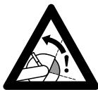
Reactive forces may occur at any time the cutting wheel on a cut-off machine is rotating. The powerful force used to cut through a workpiece can be reversed and work against the operator. If the wheel is slowed or stopped by frictional contact with any solid object or by a pinch or binding, reactive forces can occur instantly and may result in the operator losing control of the cut-off machine, which, in turn, may result in serious or fatal injury.
