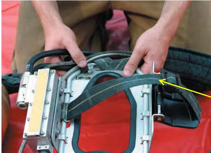
Check Harness for cracks or broken welds
