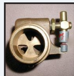
Restricts Water flow, as it is turned closed
