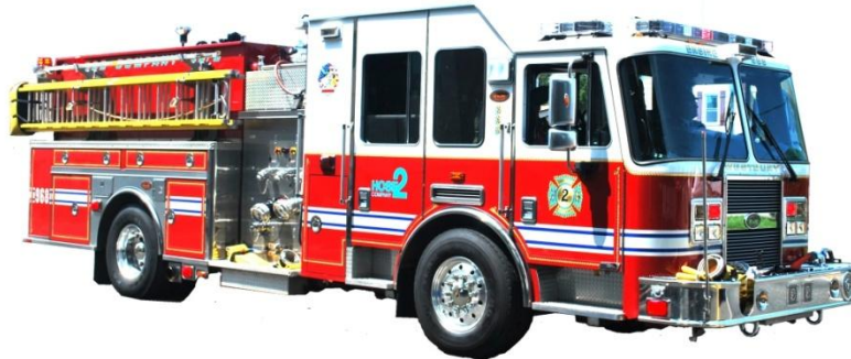
968 – KME 1500 GPM Engine w/ 600 Gal. Water
