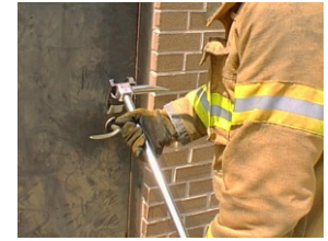
Pry Halligan Down Removing the lock from door
